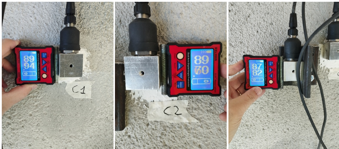
Fig. 56 Control of the sensor orientation.
