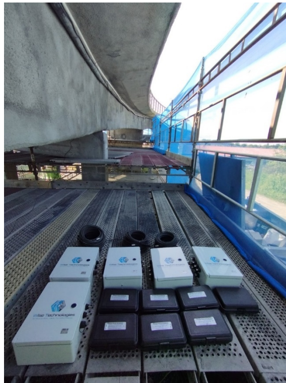
Fig. 46 Sensors and DAQ before mounting.
