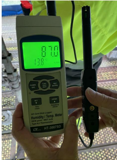
Figure E-1: Instrument used to measure moisture.
