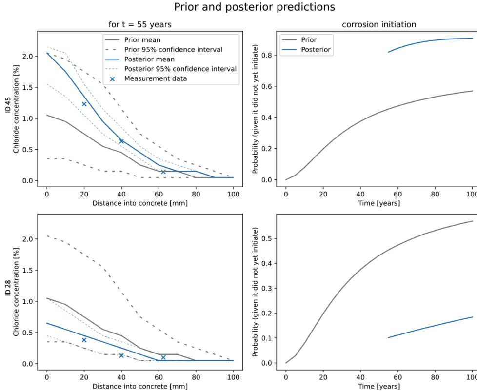
Figure 6: Updated chloride content predictions and probability of corrosion initiation over time.
