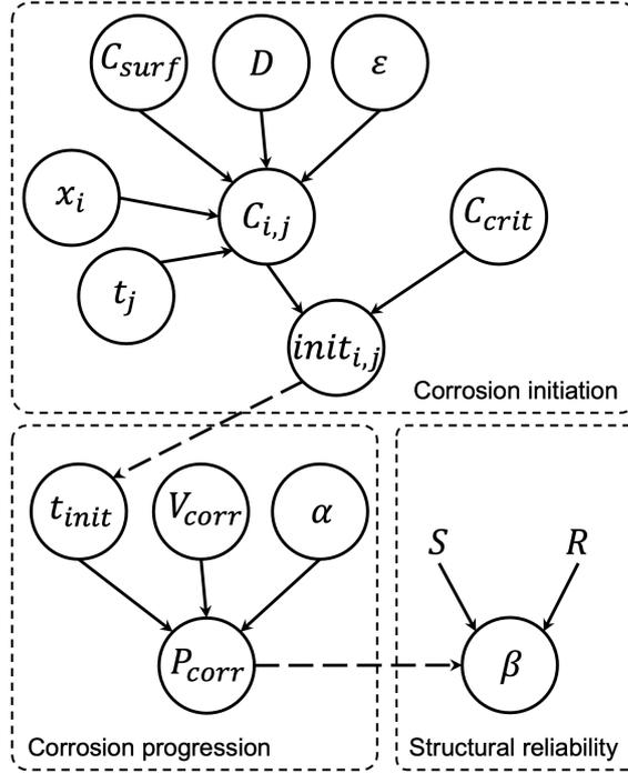
Figure 5: Structural performance modelled in a Bayesian network.
