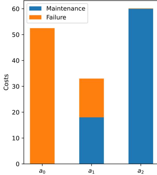
Figure 7: Total expected cost for decision alternatives: no action, minor repair, and major repair.
