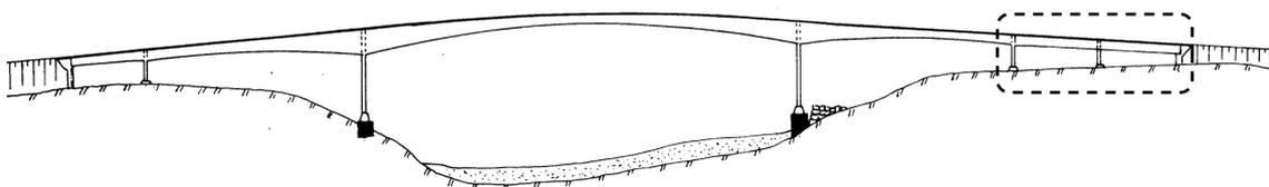
Figure 2: Drawing of Herøysund bridge. The side-spans under investigation are highlighted.
