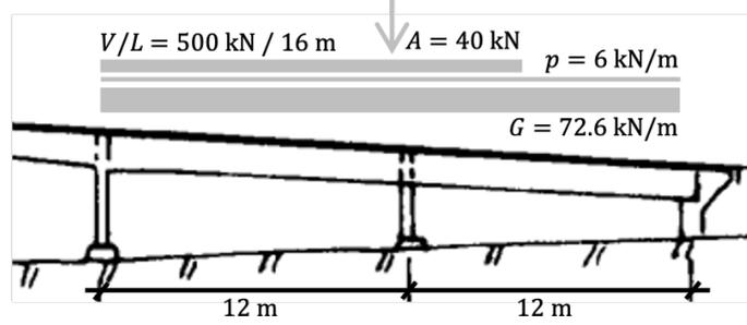
Figure 4: Governing load situation for shear with characteristic values from R412 [6].
